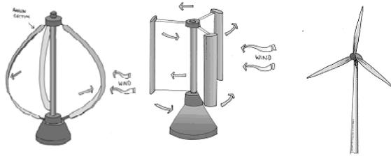
**Figure 7:** Vertical-Axis Wind Turbines and Horizontal-Axis Wind Turbine
