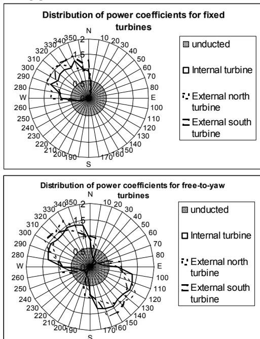
Figure 12: Power Coefficients for fixed and free-to-yaw turbines [4]
