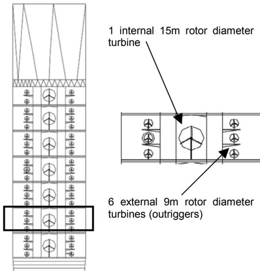
**Figure 11:** Tower integrated wind farm in tower
